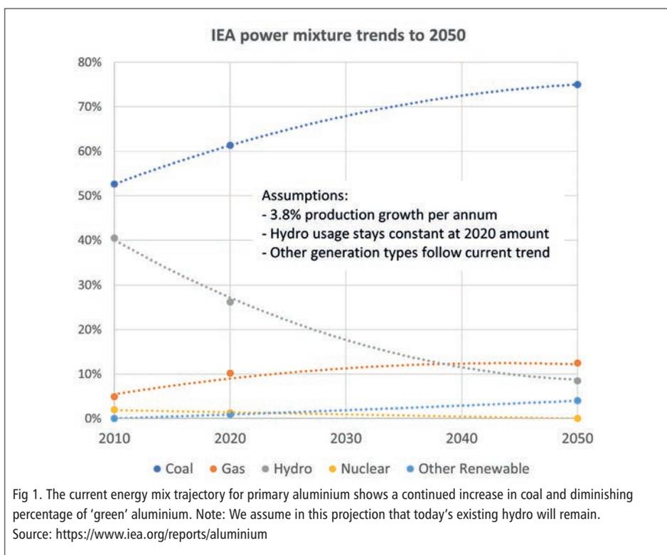
Fig 1. The current energy mix trajectory for primary aluminium shows a continued increase in coal and diminishing percentage of 'green' aluminium. Note: We assume in this projection that today's existing hydro will remain. Source: <https://www.iea.org/reports/aluminium>
